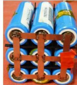
9PS1 Module with 0.5 mm Cell Spacing
